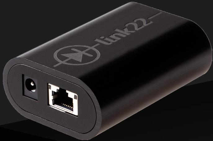
**If you are looking for a data diode with a large amount of power in a petite package at a reasonable price, look no further! Data Diode Zero can handle speeds up to 1 Gbit/s and weighs only 140g. Therefore, you can fit a large number of them into your environment.**
